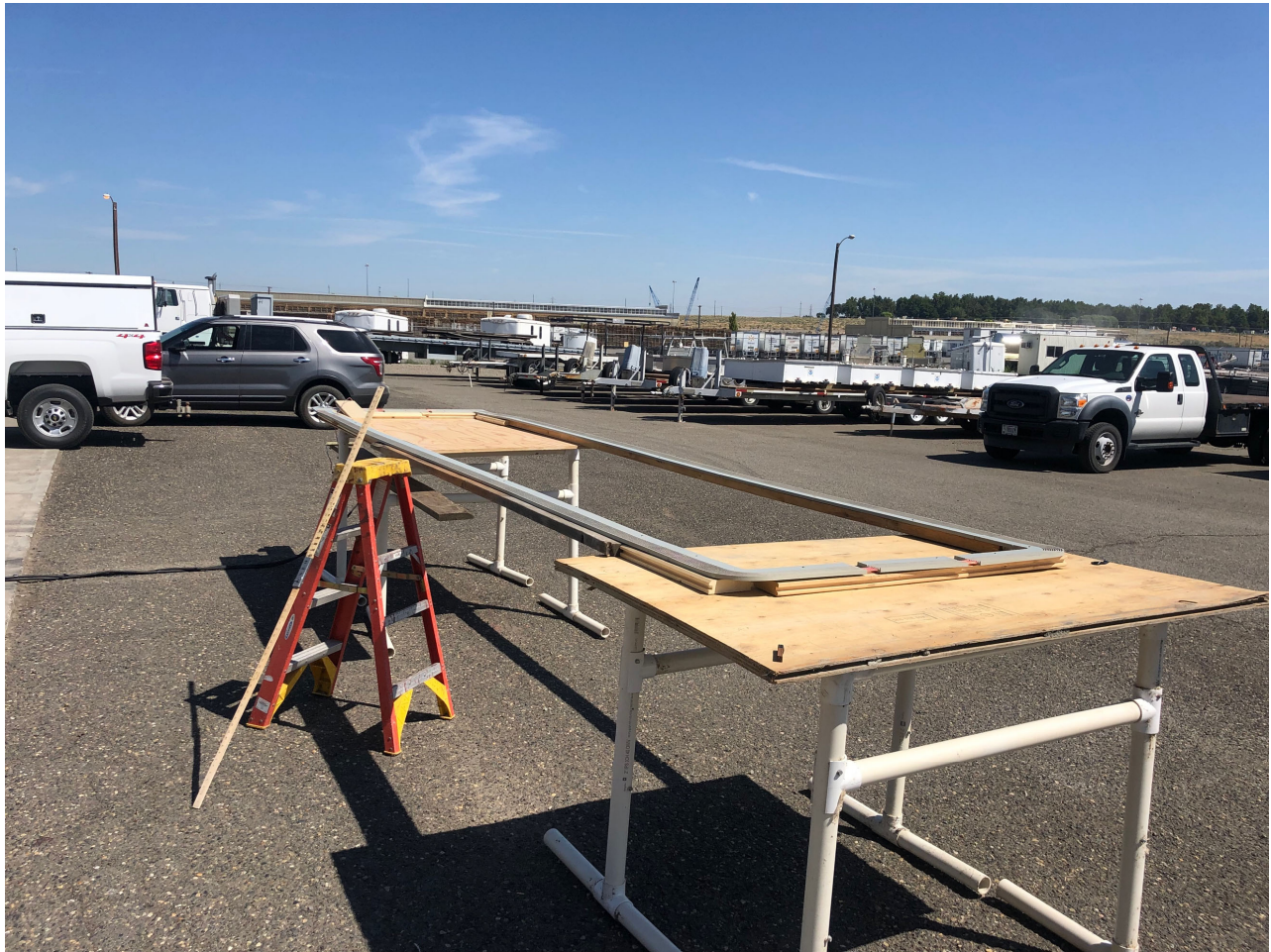
Figure 2. Test Antenna Setup Jig
